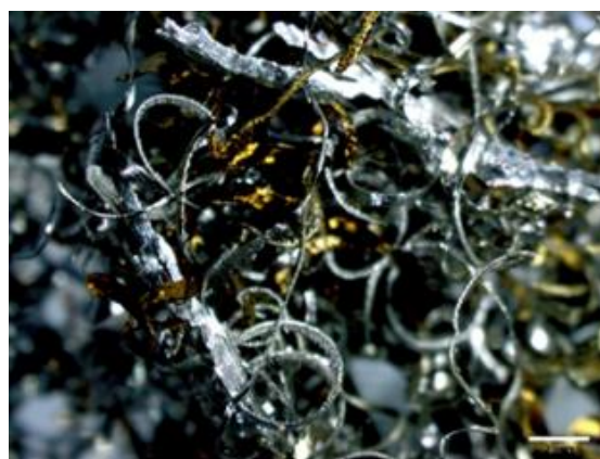
Fig. 1. AA 7075 swarf produced from the machining process
