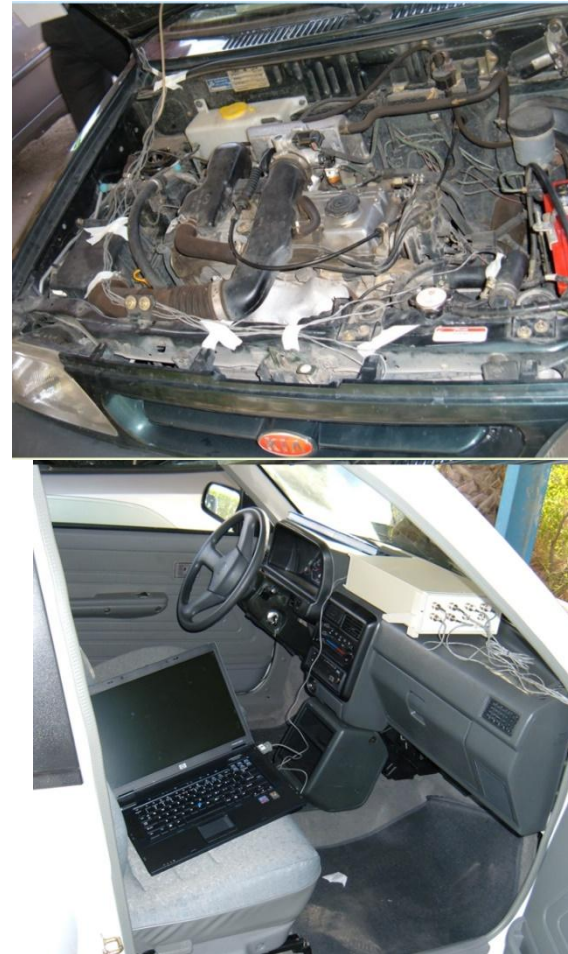
Figure 7: The data acquisition system and temperature sensors
