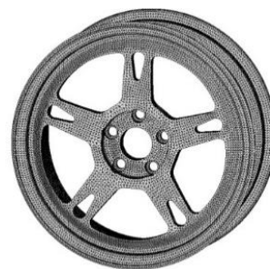
Figure 23: Re-meshed model of wheel
