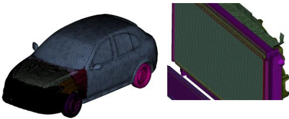
Figure 4: Surface meshing of car model and cooling system
