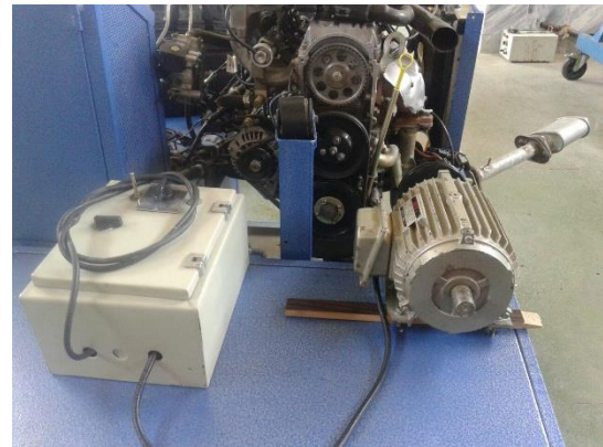
Figure 1: Motor setup, electric motor and inverter
