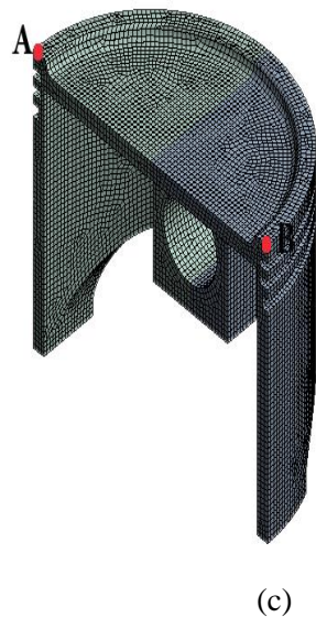
Figure 1. The piston used in the FE analyses: a) gasoline engine b) the piston, c) meshing of the FE model.
