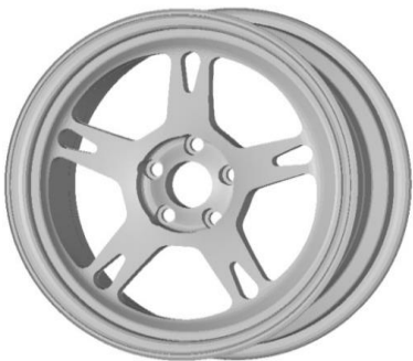
Figure 20: The optimized design after topology optimization
