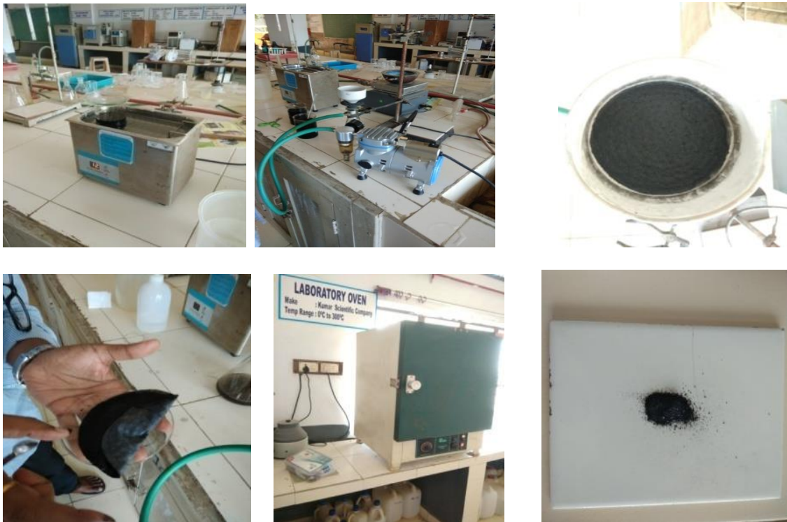
Fig 2.4.3 Sequential operations carried out in MWCNT surface oxidation to form MWCNT-F
