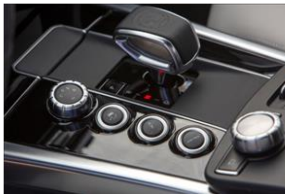
Fig5. Proper usage of texture prevents fingers from slipping
