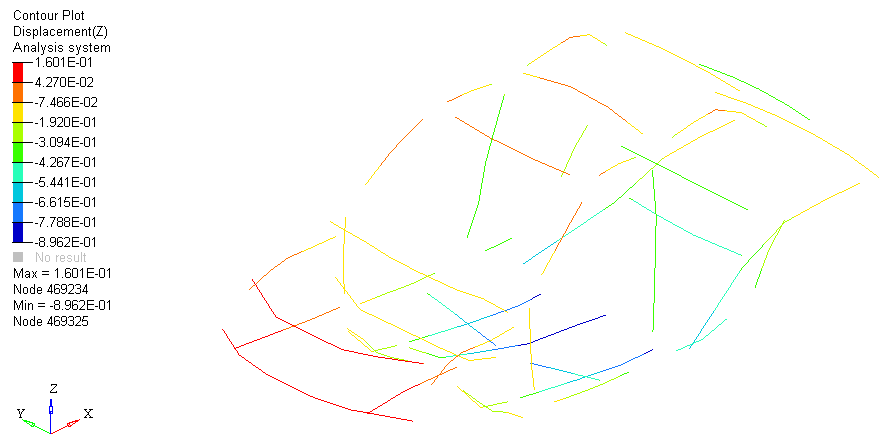
Fig5.Displacement contour of concept vehicle model in bending analysis
