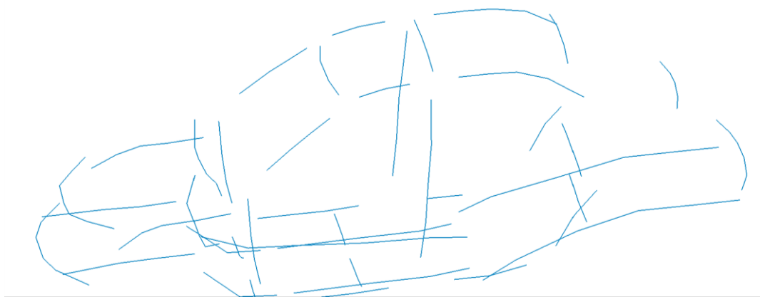
Fig3.: Equivalent beam modeling of the BIW
