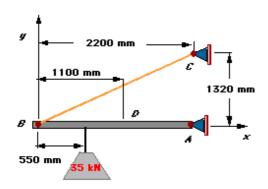
The 2.2-m-long beam  $\mathcal{AB}$  is supported by a pin at  $\mathcal{A}$  and a cable  $\mathcal{BC}$ . The beam carries a 35-kN load 0.55-m from end  $\mathcal{B}$ . Determine the absolute value of the maximum normal stress at section  $\mathcal{D}$  of the beam knowing
