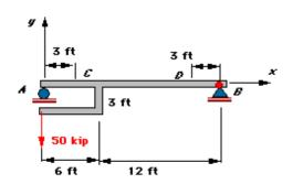
The 18-ft-long beam  $\mathcal{AB}$  is loaded and supported as shown. Determine the absolute value of the maximum normal stress at sections  $\mathcal L$  and  $\mathcal D$  of the beam knowing
