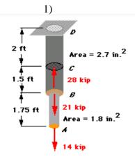
Rod ABCD is made from aluminum ( $E = 10 \times 10^6$  psi) and is subjected to the three applied forces shown. Neglect the weight of the rod, and determine the displacement of point A.
