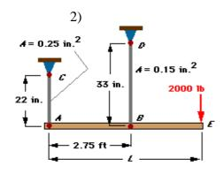
Rigid beam  $\mathcal{ABE}$  is supported by two steel rods ( $\mathcal{E}$ = 30  $\times$  10<sup>6</sup> psi) and subjected to a 2000-lb load applied at  $\mathcal{E}$ . Determine the length ( $\mathcal{L}$ ) of beam  $\mathcal{ABE}$  so that the angle formed by the beam and a
