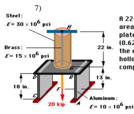
A 22-in. section of steel with a 1.375-in.  $^2$  cross-sectional area rests on a rigid platform supported by two aluminum plates (1.5  $\times$  7.5  $\times$  18 in.). A 35-in.-long brass rod (0.625-in. diameter) supports a 20-kip load at F, while the end is attached to a rigid bar (H) resting on the hollow steel cylinder. Neglect the weight of each component and determine the deflection of point F.
