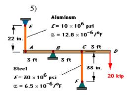
Rigid beam (ABCD) is supported by a pinned connection at B, an aluminum rod (AE), and a steel rod (EF). The cross-sectional area of both rods is 2.5 in.<sup>2</sup>. A 20-kip load is applied at D. If both rods are heated from room temperature ( $70^{\circ}F$ ) to  $170^{\circ}F$ , determine the compressive force in rods AE and EF.
