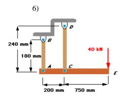
Rigid bar  $\mathcal{AEE}$  is supported by links  $\mathcal{AB}$  and  $\mathcal{ED}$ . Both links experience a temperature change of  $\triangle$   $\mathcal{F}$ = 100°C. Determine the deflection of points  $\mathcal{A}$ ,  $\mathcal{E}$ , and  $\mathcal{E}$  if a force of 40 kN is applied at  $\mathcal{E}$  and
