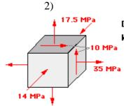
Determine the strains corresponding to the state of stress shown knowing E=200 GPa, G=76.92 GPa, and V=0.3.
