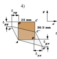
Element ABCD has dimensions of 23 mm  $\times$  30.5 mm before deforming to the element defined by ABCD'. Determine the state of plane stress required to cause this deformation knowing that E= 200 GPa, G= 75 GPa, and V= 0.33.
