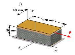
A rectangular block with  $\mathcal{B}$  = 700 MPa is bonded to two rigid horizontal plates. The lower plate is fixed, and the upper plate is subjected to a force  $\mathbf{P}$ , which causes it to move 0.5 mm. Determine the shear strain in the plate and the load  $\mathbf{P}$ .
