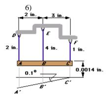
Three cables support a rigid beam  $\mathcal{ABC}$ . End  $\mathcal L$  of the beam displaces cable  $\mathcal LF$  by 0.0014 in. In addition, beam  $\mathcal AB\mathcal L$  displaces so that it makes an angle of 0.1° as indicated. Determine the normal strain in each cable.
