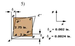
Material element  $\mathcal{ABCD}$  has original dimensions of 2 in.  $\times$  2.75 in. before deforming to the element defined by  $\mathcal{ABCD}'$ . Determine the shear strain corresponding to this deformation.
