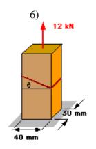
Two members with a uniform cross section of 30 x 40 mm are joined by a glued scarf splice at an angle  $\theta$ . The ultimate stresses for the glued joint are  $\sigma_{_{_{\pmb{U}}}}$  = 21 MPa and  $\tau_{_{_{\pmb{U}}}}$  = 10.5 MPa. Determine the range of values of  $\theta$  for which the factors of safety in shear and normal stresses are 2.12 and 2.8, respectively.
