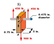
Wooden member  $\mathcal{AC}$  is supported by a 0.475-in.-diameter pin fitted into a round hole near end  $\mathcal{C}$ . For this member, determine ( $\mathcal{A}$ ) the maximum normal stress in the wood, ( $\mathcal{A}$ ) the average bearing stress in the wood, and ( $\mathcal{C}$ ) the distance  $\mathcal{A}$  required for which the average shearing stress is 90 psi along the surfaces indicated by the dashed lines.
