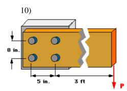
A component is attached to a wall with four 0.75-in.-diameter bolts (each acting in single shear). A load **P** is applied to the component as shown. The ultimate shearing stress for each bolt is 30 ksi. If the factor of safety is 2.5, determine the largest load **P** that can be applied to the component. *Hint*: Assume each bolt reacts the same shear force.
