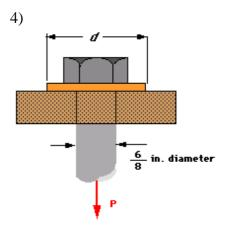
The load **P** applied to a steel rod is distributed to a timber support by an annular washer of inside diameter 0.85 in. and outside diameter d. The axial normal stress in the steel rod is 5.5 ksi, and the average bearing stress is 725 psi. Determine the required washer diameter d.
