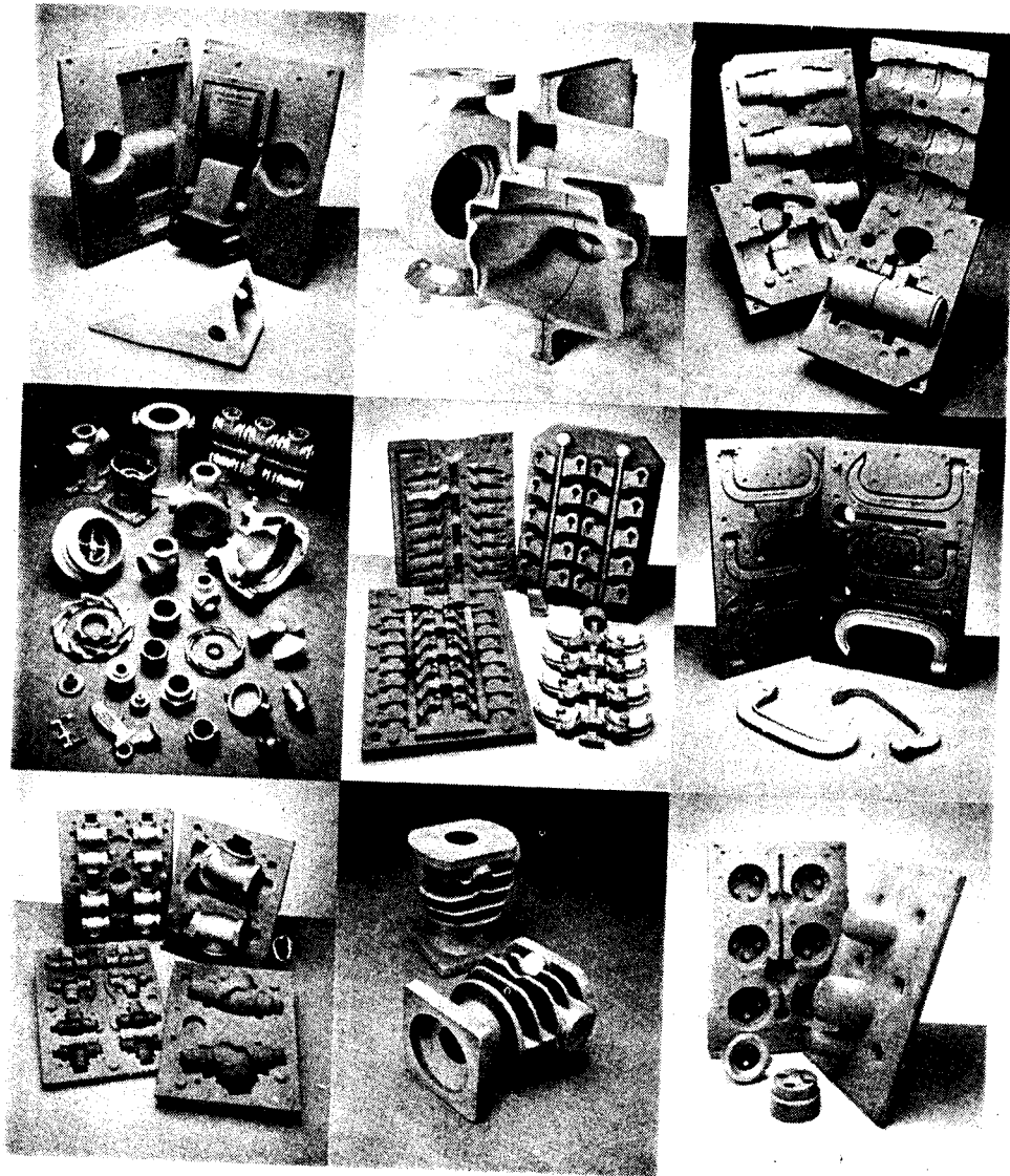
Fig. 2.20 Shell molding process
