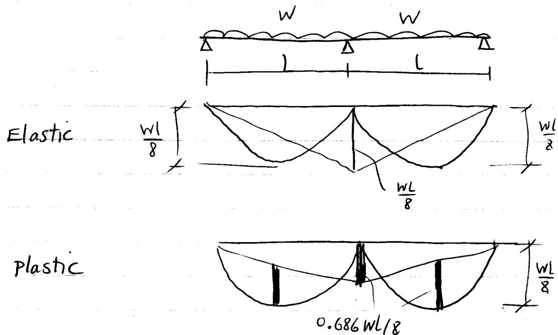
For elastic analysis,  $M_{\max} = \frac{WL}{8}$  and usually the beam is designed for this  $M_{\max}$  uniformly. It is assumed that supports do not have differential settlements otherwise  $M_{\max}$  will be reduced or increased. It is this single value on which elastic design is based.
